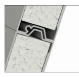
BULB SEAL Integrated bulb seal eliminates air and water infiltration keeping your interiors protected from the unwanted elements.
